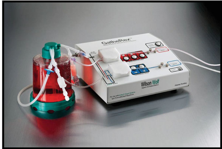
Fig. 2 The G-Rex100M-CS Cell Culture Device (REF 81100-CS) connected to the GatheRex Liquid Handling, Cell Harvest Pump (REF 80000E). The device is connected to the GatheRex using the air line attachment. The sterile weld compatible tubing (red-stripe and clear) are seated in the sensor housing that detects air bubbles which stops the fluid flow automatically once specific levels of fluid have been removed
