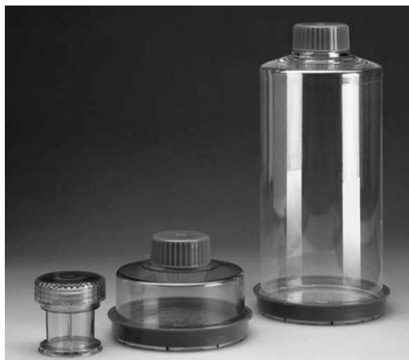
FIGURE 1. G-Rex flasks. Three types of flasks with silicone gas-permeable bottoms were used in these studies. The G-Rex10 flask has a 10 cm 2 silicon bottom and holds approximately 40 mL (left). The G-Rex100 flask has a 100 cm 2 silicon bottom and holds approximately 500 mL (center). The G-Rex100L has the same 100 cm 2 silicon bottom as the G-Rex100 flask but it holds approximately 2000 mL (right).
