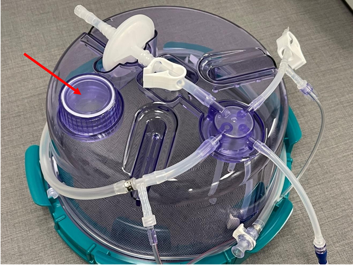
FIGURE 3: G-Rex500M-TF with removable cap
