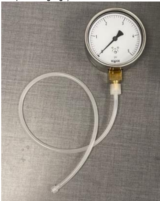
Example of pressure verification gauge assembly
